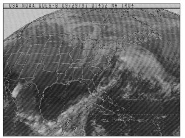
Figure 5 - GOES Co-channel interference
