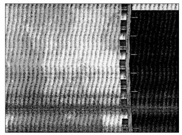
Figure 3 - Power line interference
