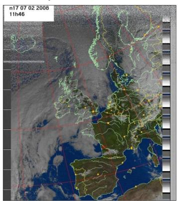
Figure 6 - Orbcomm satellite interference
