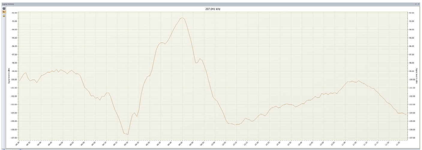
Figure 6: This is what you get if you follow the „experts“ advice: „Just look at the S-meter.“ It seems to nicely match what some people did expect as effect of the solar eclipse – a strong enhancement from the Iceland signal. But you should be warned by the near-symmetry of the trace, as the build-up of the D-layer should take more time than its vanishing. See next Figure.
