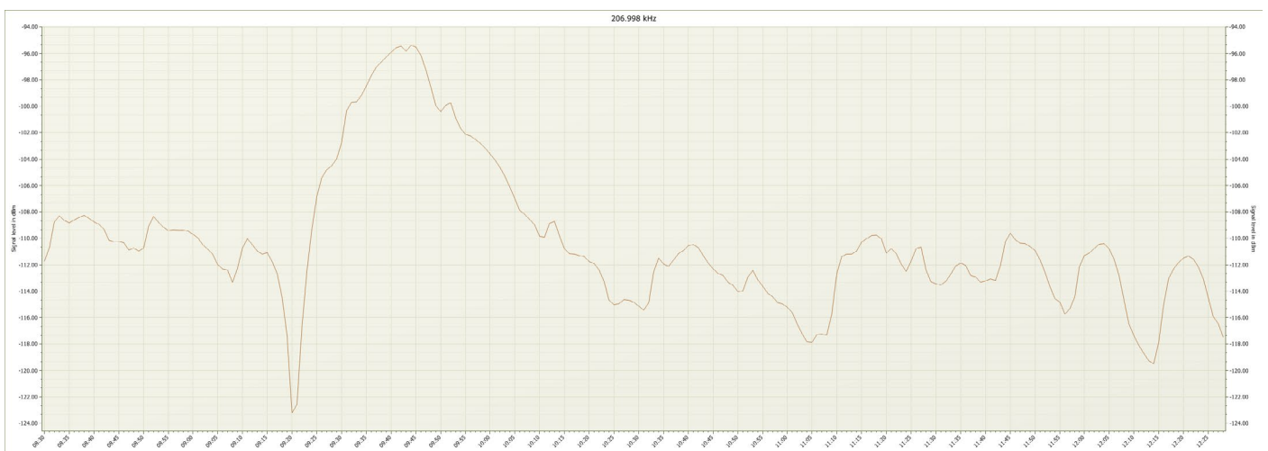
Figure 7: Here you see only the signal trace of the station from Iceland/100 kW, on the east coast of this island. The trace is not more symmetrical, but shows a steep slope in the beginning (plus an even sharper and shorter dip at 09:21 UTC when the total eclipse starts!), and a more smooth decay. Also observe the sinusoidal form of the trace from 11:40 UTC which cannot be seen in Figure 6. See next Figure for the trace of the signal from Morocco.
